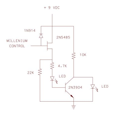
NOTE: ABOVE RESISTOR VALUES PROVIDE APPROX. 1 MA CURRENT THORUGH EACH LED, WHICH WILL GIVE CORRECT BRIGHTNESS ONLY IF SUPER BRIGHT LEDS ARE USED.
