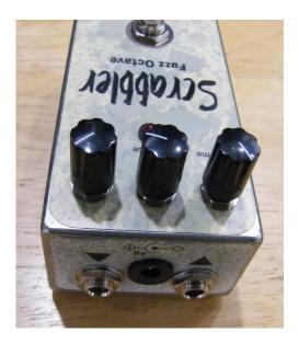
This is the Ampeg Scrambler Replica kit. This is a Fuzz/Octave unit. The Octave up sound is not as pronounced as some of the other Octave up stompboxes, but this one has a unique one-of-a-kind sound that you don't want to miss out on. This version has a transparent discrete boost stage so that a very useful Volume Control could be added. The boost stage does not alter the original tone of this effect.
