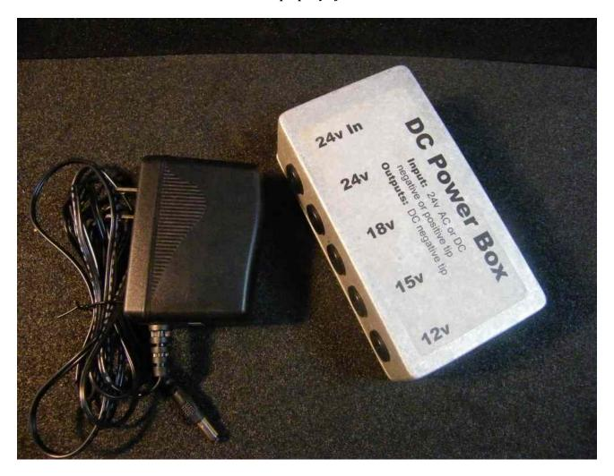
The "Power Box" also known as the "Poor Man's Bench Power Supply". Our "box" takes a 24v input and has four outputs: 24v, 18v, 15v, and 12v. This is an extremely useful tool to have on your work bench or in your studio. You can reduce the number of different wall warts you need. We only have a 24v "one spot" type wall wart and a few 9v regulated wall warts in our studio now.
