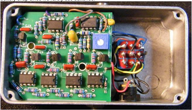
Here are voltage readings taken from our prototype unit. The voltage on the Gate of the JFETS moves around some. Put the speed on lowest setting (full counter-closewise).
