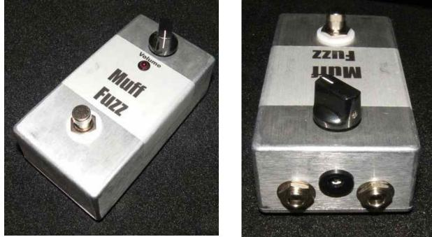
This is a **Electro-Harmonix<sup>™</sup> Muff Fuzz<sup>™</sup>** Fuzztone replica known here as the **EMTR** Fuzz. This is a very simple kit to build. Follow the Bill of Materials, the Layout diagram and General Build Instructions.
