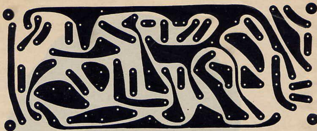
Fig. 2. Actual size printed circuit board etching and drilling guide is shown above. At right is components placement and orientation guide. Note orientations of flats on transistors and plus sign on rectifier assembly.
