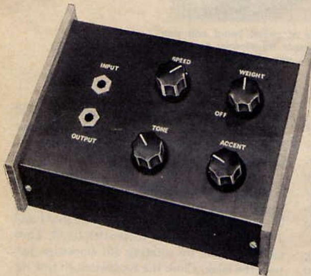
In prototype, top of case slopes downward. Top, front, and rear panels are painted flat black to contrast with rich tones of walnut side panels. Controls and jacks are lettered in white, using dry-transfer lettering kit.
