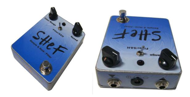
This is a replica of the *Maestro Filter Sample/Hold*. Referred to as **FSH** in these documents. This exact circuit with the same PCB and enclosure (with different graphics) was also released as the *Oberheim Voltage Controlled Filter*. Both were released in the mid to late 1970's. This pedal has a great Envelope Follower Filter (sometimes known as voltage controlled filter or auto wah) and has a cool Sample/Hold (S/H) setting as well.
