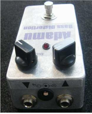
This is the Adamu Bass Preamp or Distortion. Use the project documents provided, starting with the General Build Instructions. Make sure the polarized capacitors are installed correctly according to the layout/wiring diagram. Note that there are several blank spaces for components since this is a "Multi-Use" PCB. That is okay, just follow the layout/wiring diagram and the photo below.
