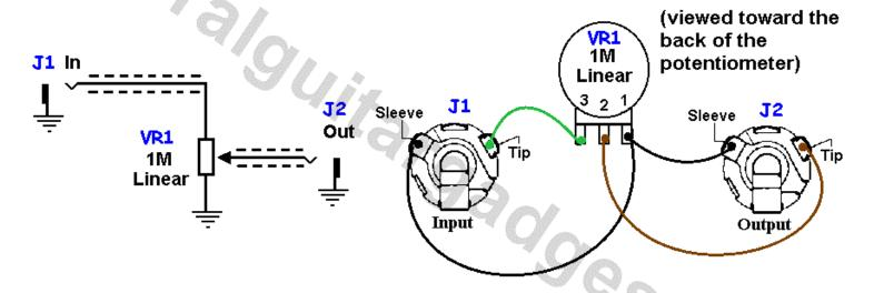
The 1 Meg pot is shown as you look at the back of the pot. The pot has a plastic pinion and the pedal has a plastic rack, similar to the "Crybaby wah wah pedal. The wiring is shielded wire with the shield connected at the "sleeve" of the jacks on one end, and at lug 1 of the pot on the other end.
