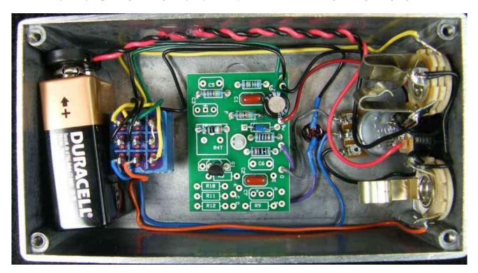
Here's a view of what it looks like with the 1590B (smaller box) option. Note that you don't use the plastic PCB standoff, you use some double sided tape and set the PCB on top of the back of the pot.
