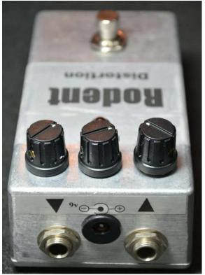
This is the Rodent Distortion kit, a replica of the ProCo™ Rat™. There were/are several versions of the Rat™. This project and kit is based on an older version of the Rat™ circuit sometimes known as version "B". It does not include a JFET on the input of the circuit as version "A" had. Experimentation has shown the input JFET does not have much effect on the sound and is probably not worth the extra parts to include it in this project.
