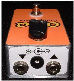
This is a replica of the **Dan Armstrong**<sup>™</sup> **Orange Squeezer**<sup>™</sup> **Compressor** referred to as **OSQ** in these documents. This Compressor doesn't have all the controls of some of the other compressors, but it's got a very nice compression sound that is not completely attainable from the others.
